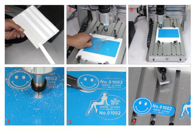
There is a file in the "tool path for machine test" of the random CD, with the file name of "shuangseban.nc". The area of this engraving file is about 75\*85mm. Because the double color plate is pasted on the auxiliary operating platform, the size of the material should within the scope of 90X90mm. Meanwhile, the initial point of this file is on the top left corner.
