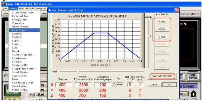
Please carefully read the above picture for setup, and the mistake of any number or option will lead to the failure of the engraving machine, or even lead to accident when operating the machine.
