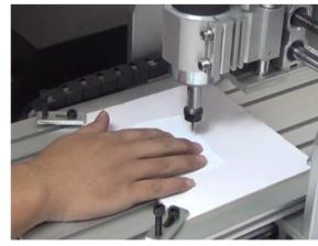
①First, we operate the XY axis through manual control, and move the principal axis close to the initial point; Install a flat base pointed knife.
